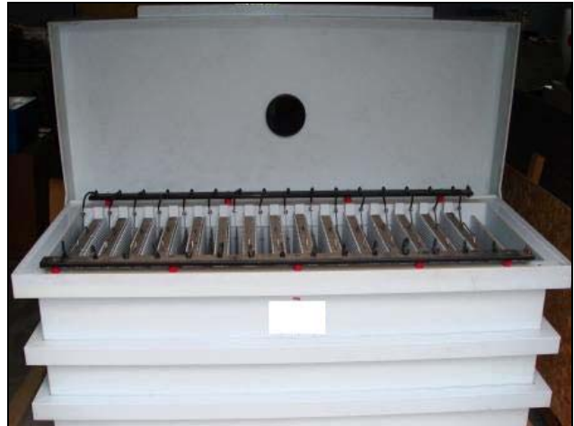
EW cell with 15 cathode boxes and 16 anodes
