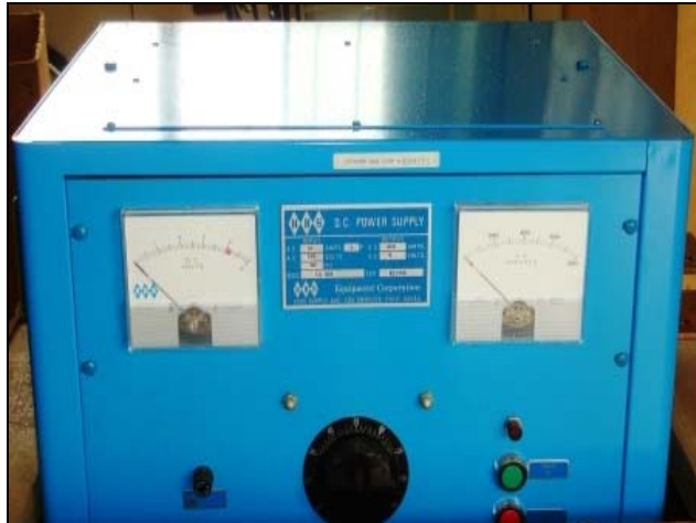
0 to 800 A and 0 to 4 V rectifier
