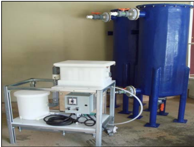
Gold EW pilot plant with carbon columns
