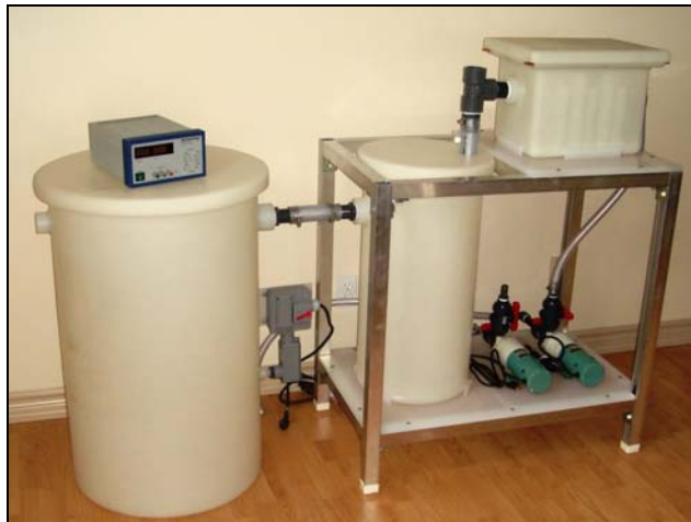
Gold EW pilot plant with 5 A rectifier
